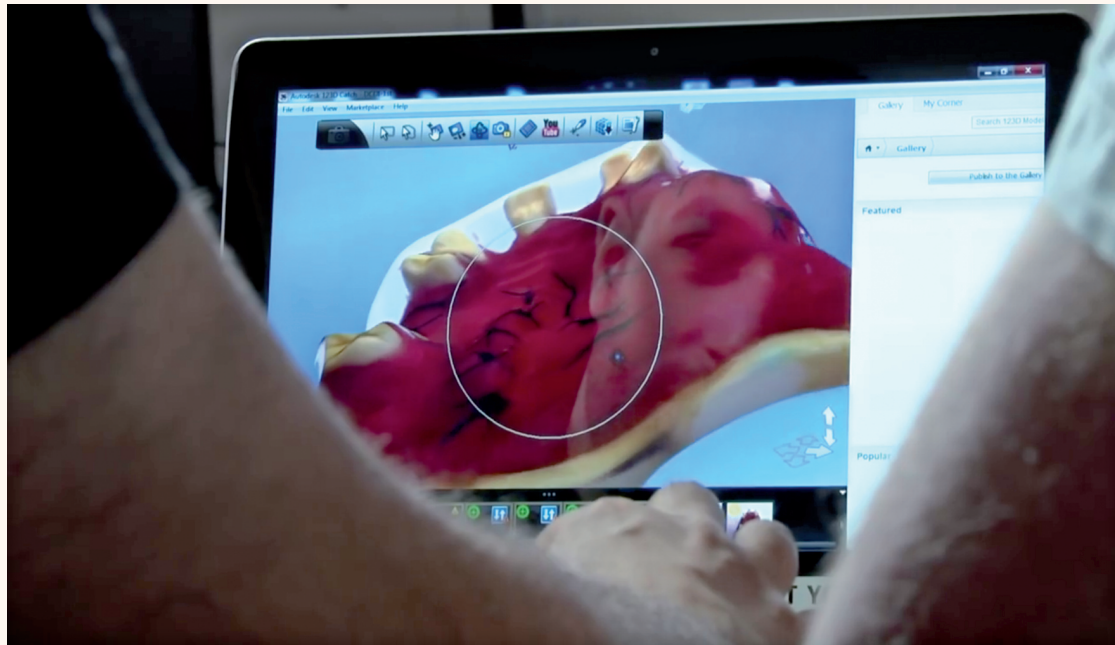
The 3-D scanner produces a precise digital impression of the mouth and outputs it to a computer, reducing the time it takes to get dentures from 30 days to 30 minutes. (© Hebrew University of Jerusalem/Hadassah Medical Center; Screenshot/DTI)
