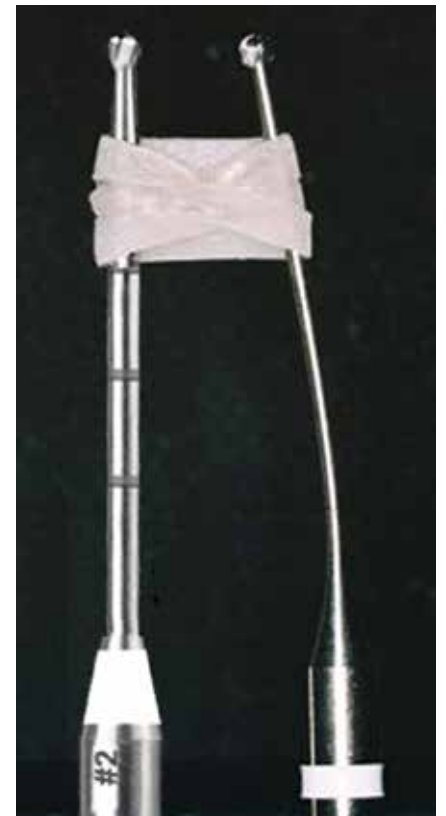
Fig. 5: Stiffness of Munce Bur shaft v. noodling of Mueller Bur shaft.
