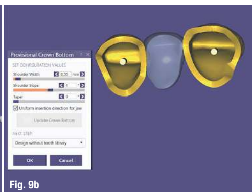
Case 2—Figs. 9a & b: Positioning of the insertion angle of the future preparation (a). Adjustment of the thickness of the walls of the temporary bridge (b). Fig. 10: Temporary FDP milled (dentallgroup.eu).
