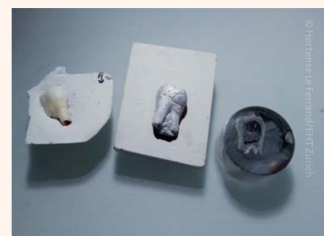
Natural tooth in its gypsum mold, artificial tooth (sintered but not yet polymer infiltrated), finished artificial tooth embedded in a "puck" to enable polishing.
