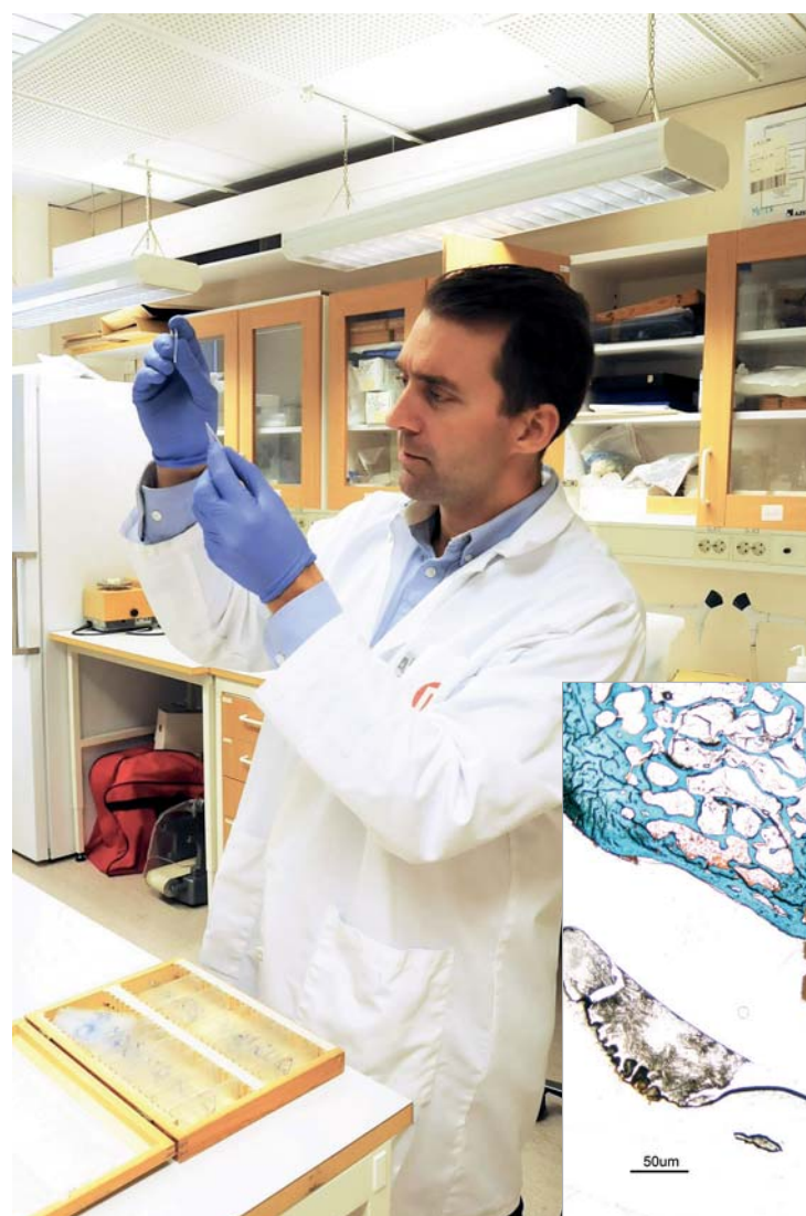
*Dr Johansson is examining histological sections of the implant in rabbit bone before looking at this in the microscope. This is a histological image from a PEEK implant with a hydroxyapatite coating. This one is implanted into rabbit bone and retrieved after three weeks of healing. At the bottom of the implant you can see the osteoconductive properties of hydroxyapatite on PEEK as the bone bends and grow along the implant surface.
