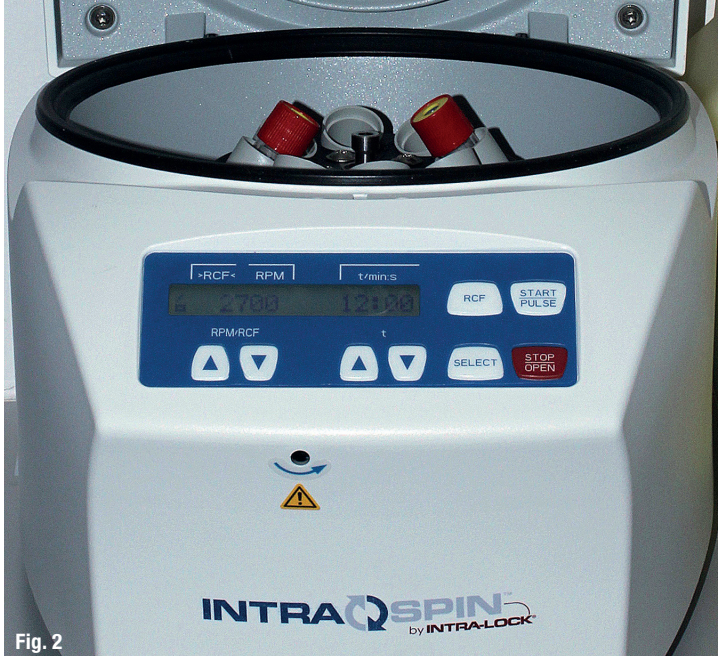
Fig. 2: Centrifugation at 408 g RCF, (2,700 rpm) with IntraSpin™ centrifuge. Fig. 3: L-PRF clot in tube; clear separation: red blood corpuscles (RBCs) at the bottom, PPP (platelet-poor plasma) on the top, and L-PRF fibrin clot in the middle.
