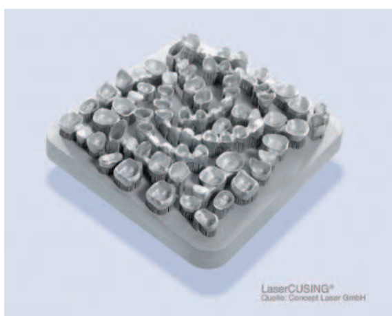
Crowns and bridges manufactured using laser melting technology.
