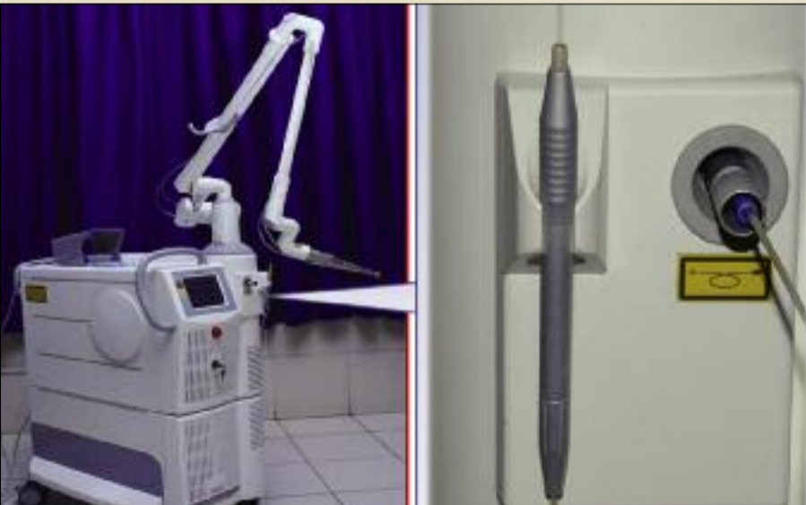
Fig. 6a: Nd:YAG laser from Fotona with 200 μm fiber has also been tried for gutta-percha removal.
