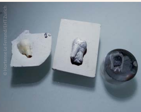
Natural tooth in its gypsum mold, artificial tooth (sintered but not yet polymer infiltrated), finished artificial tooth embedded in a "puck" to enable polishing.
