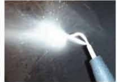
SE15 Handpiece With ST 106 Serrated Cutting Tip
