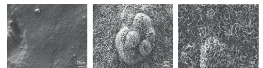
Left: Predicta Control, no SBF. Center: Predicta, 7 days in SBF. Right: Predicta, 28 days in SBF. SEM images courtesy of Håkan Engqvist, Uppsala University, Sweden.
