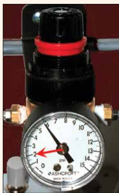
Fig. 7. The Chapman-Huffman in-line air regulator and 0-15 psi gauge works well.
