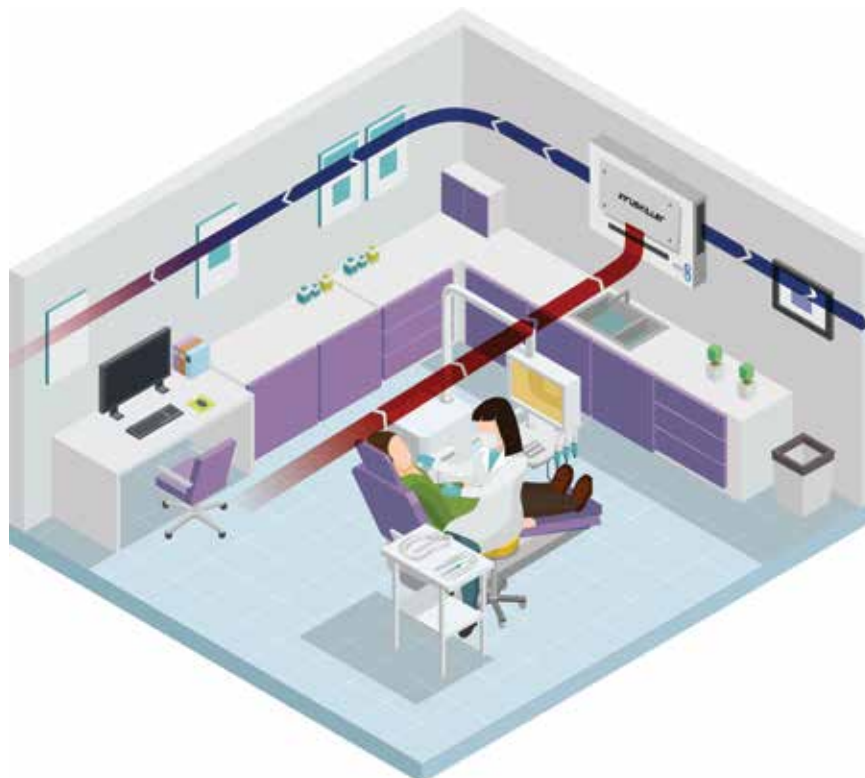
• The VK 401 is designed for operatories. When properly positioned, it can draw air away from the breathing zone, through the VirusKiller Technology and then sending purified air laminarly along the walls and into the breathing zone. (Photos/ Provided by Henry Schein)
