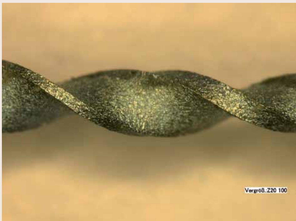
Fig. 6_Surface of the HyFlex EDM under the microscope.
