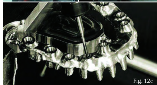
Figs. 12a-c Machining from a titanium block.
